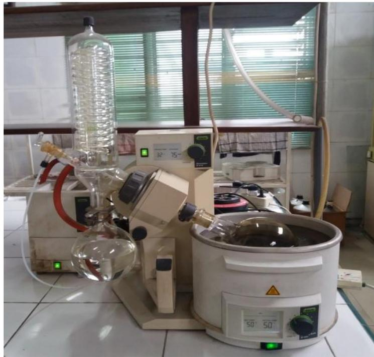
Gambar 3. Alat Rotary Evaporator
