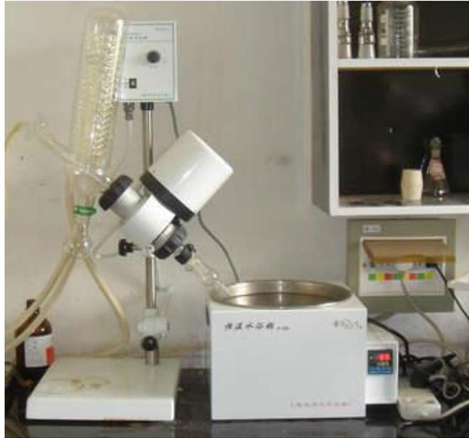
Gambar 3. Alat Rotary Evaporator
