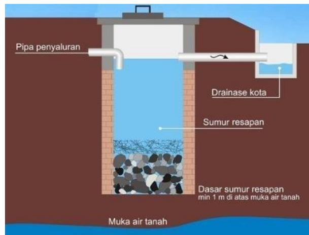
Gambar 2.5 Sumur Resapan (Kumpul Engineer)
