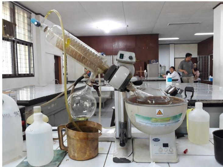
Gambar 5. Rotary evaporator
